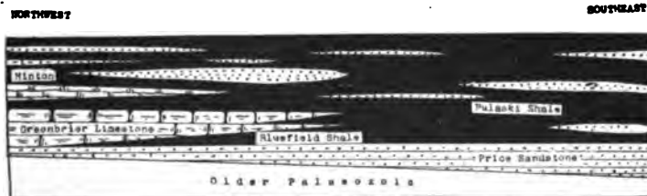
FIG. 1359. — Ideal section showing the interpretation of the relationships of the several Mississippian formations in northeastern Virginia. The Pulaski shale on the east (black) contains many sandstone lenses, white and dotted, and represents the near-shore end of an ancient delta-like deposit. The beds are very variable in color and other characters, indicating a subaërial origin, i.e. the exposed part of the delta. The beds are about 3000 feet thick in the east, thinning away westward. (Modified after Branson.)
